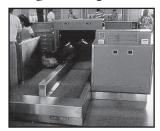
Increasing demands for security scanning belts have increased the need for a non-metallic splice. The Alligator® Spiral Lace is a low-profile, non-marking, hinged splice that is ideal for security belts. Alligator Spiral Lace is vulcanized into the belt by belt fabrication shops. Available in a variety of sizes and either black or white materials.
