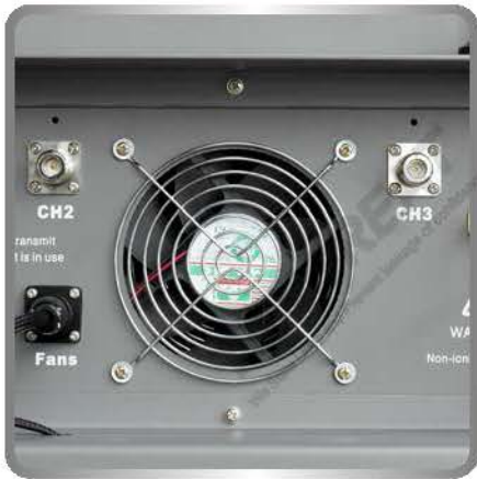
Active Cooling System
