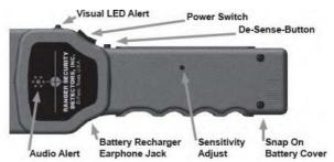
The metal detector has an automatic system calibration and the ability to adjust the sensitivity, ensuring optimal performance for applications in weapons detection and prevention.
