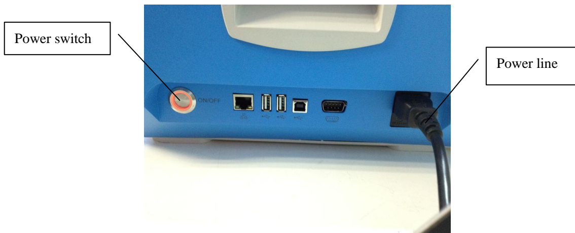
Figure 10 Power supply and power switch
