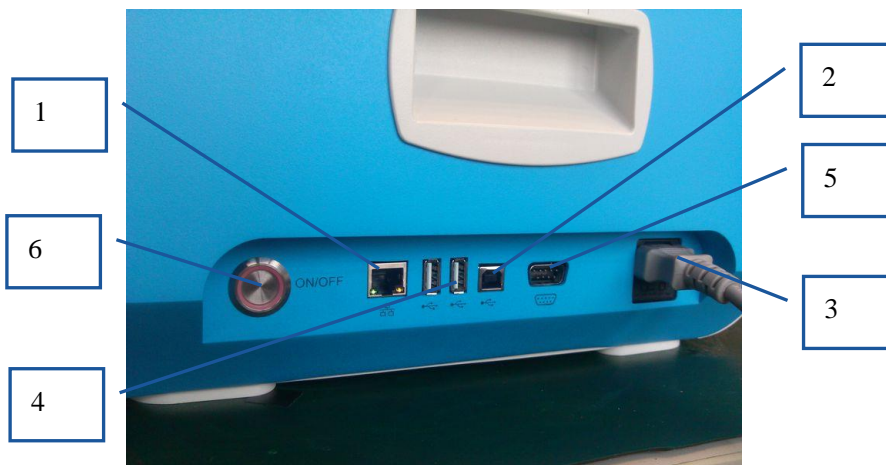
1 RJ45 network interface used for network transmission, 2 Type B USB interface used for equipment support, 3 Power cord, 4 2-off Type A USB interfaces used to connect external USB devices such as a USB keyboard, mouse, or USB disk, 5 RS-232 interface used for peripherals such as a printer; 6 Power switch.
